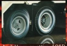
Available as an option, LOAD-MASTER's tag axle lowers into place to help shift weight to the front axle, increase load-carrying capabilities and help reduce the risk of overload fines
