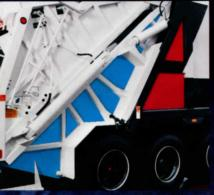
The entire hopper area (blue) is constructed of 100,000 psi high-tensile steel for greater strength and a more durable long life. The ten-gauge, high-tensile reinforced steel rear panel makes for even greater strength in the critical compaction area (red) of the body.
