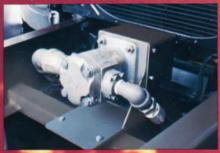
Another LOADMASTER option: Front pump system replaces the standard PTO. Eases maintenance, gives more positive pump engagement.
