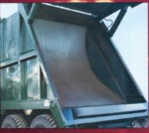
"Back-pack" valve automatically adjusts ejector blade to keep optimum pressure for more efficient, uniform loading.
