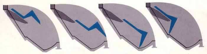
Operator starts packing cycle. Packing plate automatically moves upward. Packing plate moves to rear over top of fully loaded hopper. Packing plate clears refuse from hopper.
