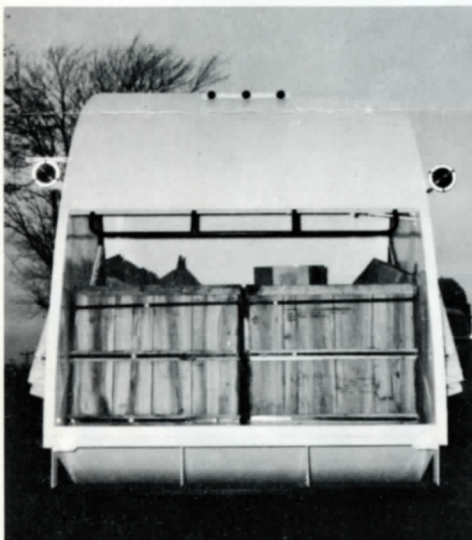
Large capacity Hopper takes two cubic yard load of bulky materials with ease. Start reloading in seconds.
