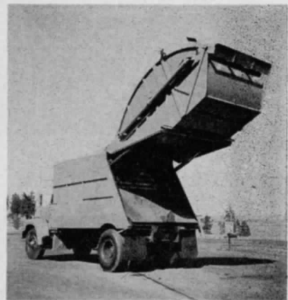
Rear view of the Load-Master refuse packer, with rear of unit raised and ramrod ejector panel at the full ejection position.
