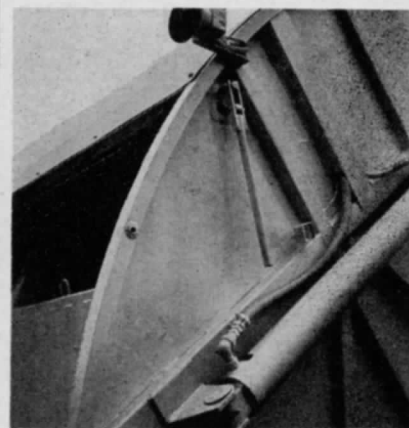
Close-up view of the Load-Master single control lever at the rear of the batch packer unit. Touch of a master lever starts the packing cycle.
