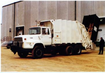
LARGE 2.3 CUBIC YARD HOPPER HAS SUPERIOR LOADING CAPACITY MTM's PACSTAR-RL allows for much faster collection and fewer compaction cycles on route. (Optional 2.8 cubic yard with a 5" Hopper Extension).
