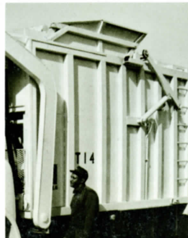
Patented hydraulic actuated compaction cover lifts and slides back for loading. Once open, cover need not be closed until heavy compaction begins; saves valuable minutes per stop.
