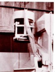
Special loaders can be provided for dumping 55 gallon barrels into compaction hopper, single lever controls both clamping and lifting.
