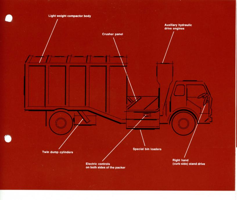
Right hand (curb side) stand drive assembly adds valuable minutes to the efficiency of a one man operation. Factory controls for left hand drive are retained to insure standard safety during normal highway travel. Crusher panel crushes material into hopper before packer blade pushes it into body; speeds compaction of items such as tree trimmings, wooden crates and boxes.
