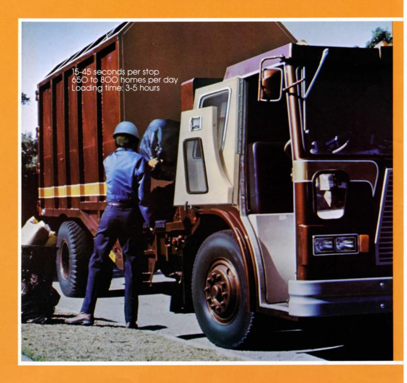
SIDE LOADER BODY, REFUSE CAB & CHASSIS BUILT AS AN INTEGRATED UNIT
