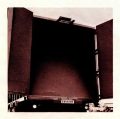
The Full-Pak's packer plate extends to the end of the body and floor for clean load ejection. Packer plate guide channels are mounted in the corner of the floor and sidewalls, not down the middle of the hopper where the blade can become untracked or sprung.
