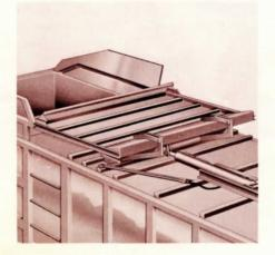
Optional compaction cover hydraulically lifts and slides back for loading, like a sunroof instead of a trap door. You get a lower, safer profile. And the cover doesn't have to be closed until heavy compaction starts, so you save more time. Unlike hinged covers which can be sprung easily, the Full-Pak's patented cover drops down on top of the load as it closes. You never have to shear through trash because nothing can get between the cover and the hopper.
