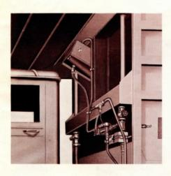
The 70-gallon oil reservoir is an integral part of the front wall structure which eliminates expensive chassis modifications. You get better weight distribution and reduced overall weight. Double tank construction provides excellent heat dissipation.
