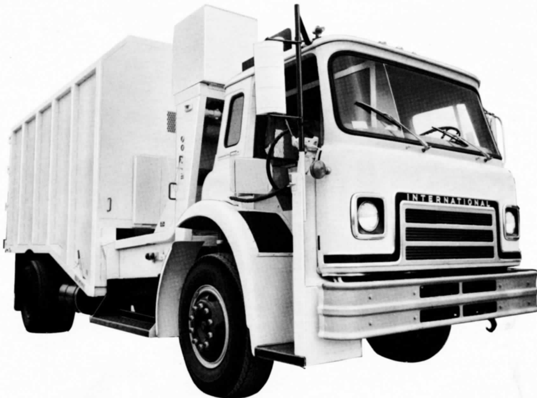
Cab partition provides normal driver comfort in colder climates.
