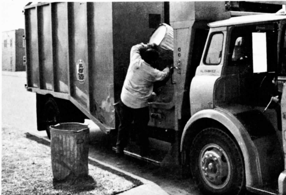
Ford 172-powered, Shu-Pak compactor-equipped truck can be operated by one man in a right-hand, stand-up cab moving from load to load
