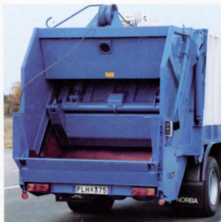
The wear surfaces of the packer plate, like those of the hopper, consists of high-strength wear-resistant steel
