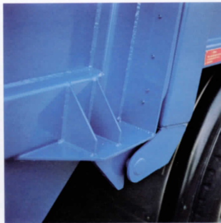
The automatic locking mechanism secures the tailgate against the body
