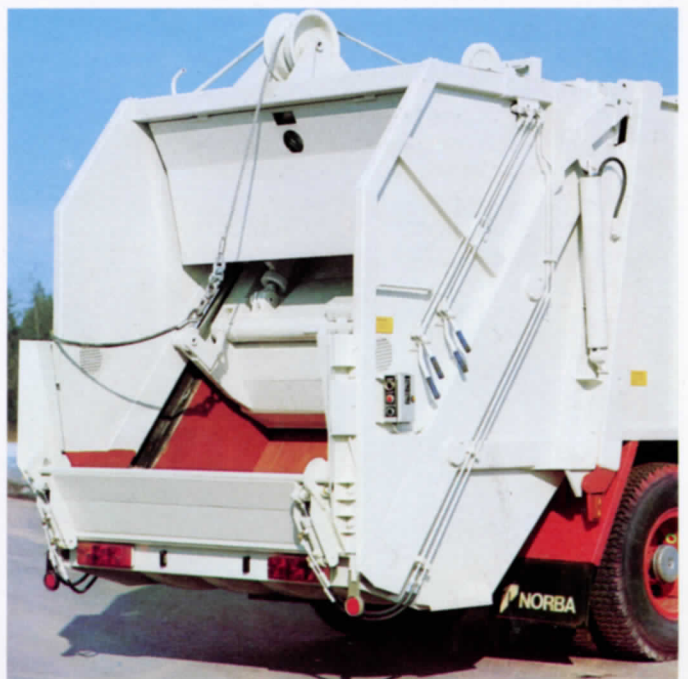
Lift for containers up to 8 m 3 with agitator.
