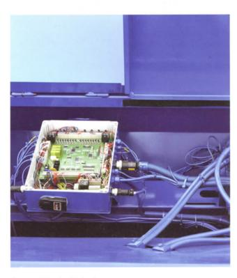
Fast and fuel efficient. Our exclusive Smart Pack System™ enables control of binlift speed and other functions, independent of loading weight. It automatically senses how much pressure the system needs to lift and pack. The result? The industry's fastest packing cycles. Plus impressive fuel savings.
