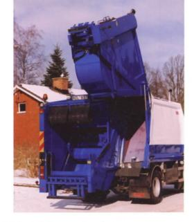
Two completely sealed compartments keep your fractions seperated without any risk of cross contamination. Each compartment has its own compaction mechanism and ejector plate, for independent loading and discharge of the fractions.
