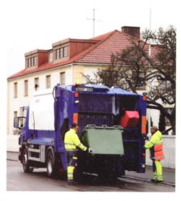
The L500 MF lifting device is specifically designed for the MF300 tailgate and provides split, independent emptying of bins. Plus it has a low rear overhang, is easy to operate and very fast. That's efficiency that leads to lower operating costs.
