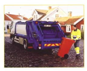
Small outside dimensions make the Norba RL 50 ideal for low passages, narrow roads and bridges, places where standard refuse vehicles can't reach. The compact design is perfect for use with chassis cabs of 7,500 kgs G.V.W.
