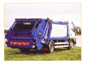
The Norba RL 50 features an impressive capacity, and offers many of the same capabilities as our standard RL series – including Our exclusive Smartpack™ system which enables control of binlift speed and other functions, independent of loading weight. It automatically senses how much pressure the system needs to lift and pack, yielding the industry's fastest packing cycles. Plus impressive fuel savings.
