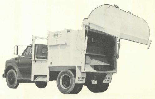
AUTOMATIC, HYDRAULIC TAILGATE LOCKS — Tailgate unlocks, raises, lowers and locks by a single control at front of packer. Initial cylinder movement releases locks, then completely opens tailgate in a single, smooth operation. No wasted time with manual levers or cranks.
