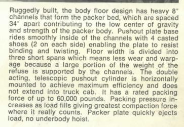
New Way engineering allows the push out plate to retract to the forward end and serve as the front of the packer body. This space saving feature permits easier maintenance and cleaning, eliminates dead weight and improves weight distribution.
