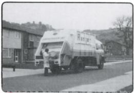
The Ranger is manufactured in four body sizes, with an air space of 10, 13, 17 and 20 cubic yards. The efficient proven compaction mechanism, together with the specially shaped ejector blade, ensure maximum payload within legal operating requirements.
