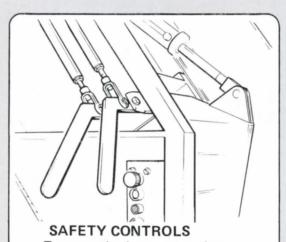
Two operation levers mounted at rear nearside of loading hopper giving split cycle operation with reversing mechanism giving full protection to operators.
