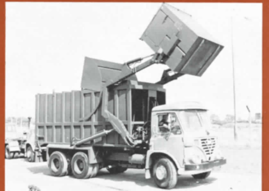
Lifting continues until the container is above the cab and Dumpmaster body.
