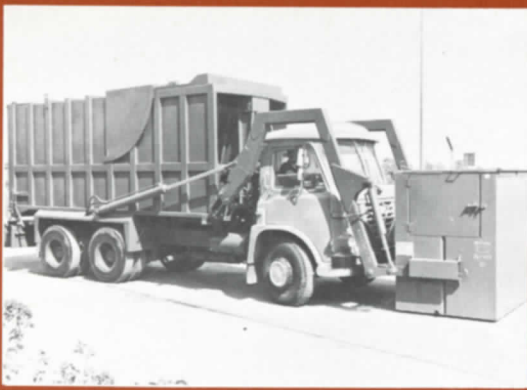
Anti-Scatter guard in open position
