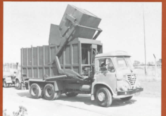
When the container is above the loading aperture, by selecting the correct control lever the container is inverted and its contents discharged into the Dumpmaster body.
