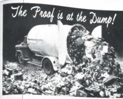
With PAK-MOR, each pick-up . . . can by can . . . is broken down to the smallest possible mass by the Packer Plate's tremendous Direct Compaction Force. This compressed mass is retained throughout the body in a series of dense layers by Finger Stays—PROOM Becouse more refuse is houled to the down in each PAK-MOR load.
