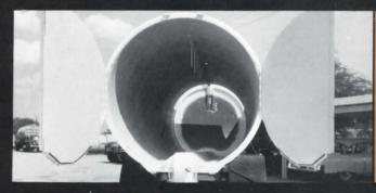
Finger stays along top of barrel provide positive load retention. This feature makes for denser and heavier loads allowing Pak-Mor to cover longer routes in a single load.
