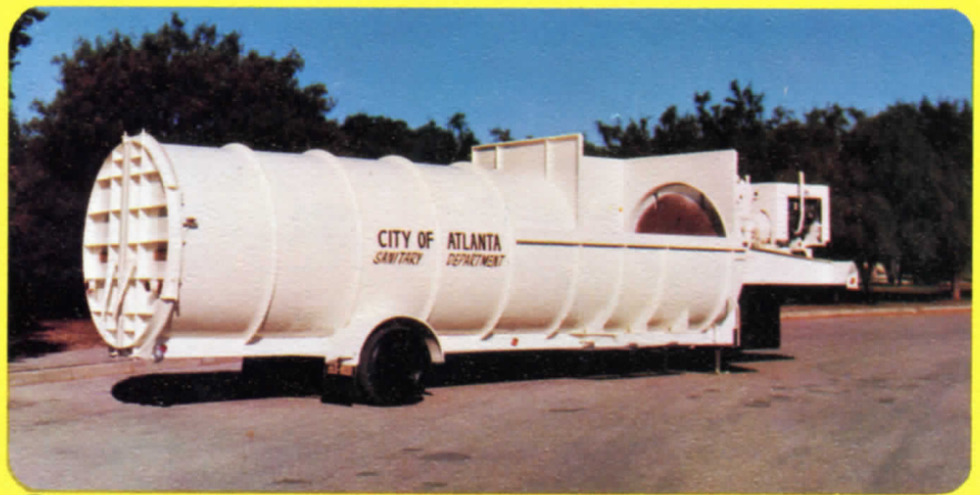
11 Large custom designed hopper to accommodate bottom discharge containers and for transfer facility operation — maximum flexibility.
