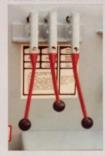
Positive lever controls are located on the streetside and the curbside of the body. The controls actuate the packer and rear door. The chassis engine throttle is automatically actuated to accelerate the engine to the proper RPM level. Available as an option are pushbutton packer controls that can be installed in addition to the positive lever controls.
