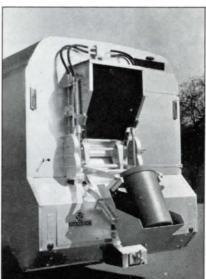
Single unit available on TN series. Single or Twin units on the remainder of the range can be used in conjunction with standard household bins or special dustless type bins with hinged lids.
