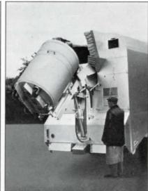
Available on all models other than the TN series. The squeeze-clamp action allows the handling of any 1 or 1½ cubic yards elliptical or circular container with bodies to standard B.S. specifications.
