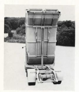
The highly successful tipping subframe which has been an exclusive feature of all **SD** Fore and Aft Tippers has been retained and still embodies the method of pivoting the body on large diameter heavy-duty roller bearings when tipping forward, and this built-in factor of safety cannot be over-emphasised.
