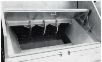
Only the outer surfaces of the packer unit are in contact with the refuse. The loading cycle continues without interruption, being fully automatic and foolproof in operation.
