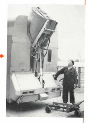
A variety of wheeled-type Containers can be lifted with equal facility, in every case the method of attachment being automatic, requiring no clamping bands or other devices; thus the **SD** Pakamatic can operate successfully with containers at present used with any other system.
