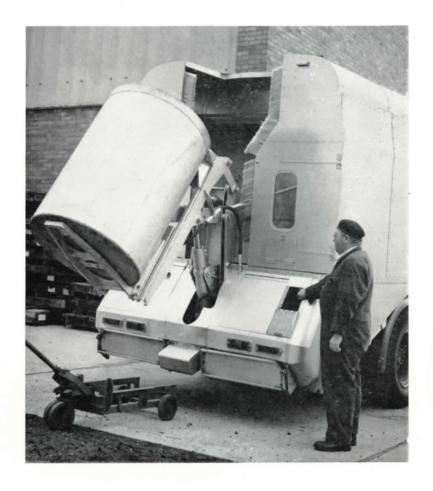
WITH PATENTED SQUEEZE CLAMP TYPE
