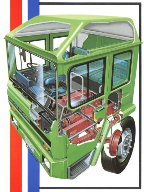
COMFORT, safety and style are built into all Shelvoke Dempster cabs. The welded steel construction with fibreglass roof canopy provides all-round safety, while the deep windscreen and windows give all-round vision.
