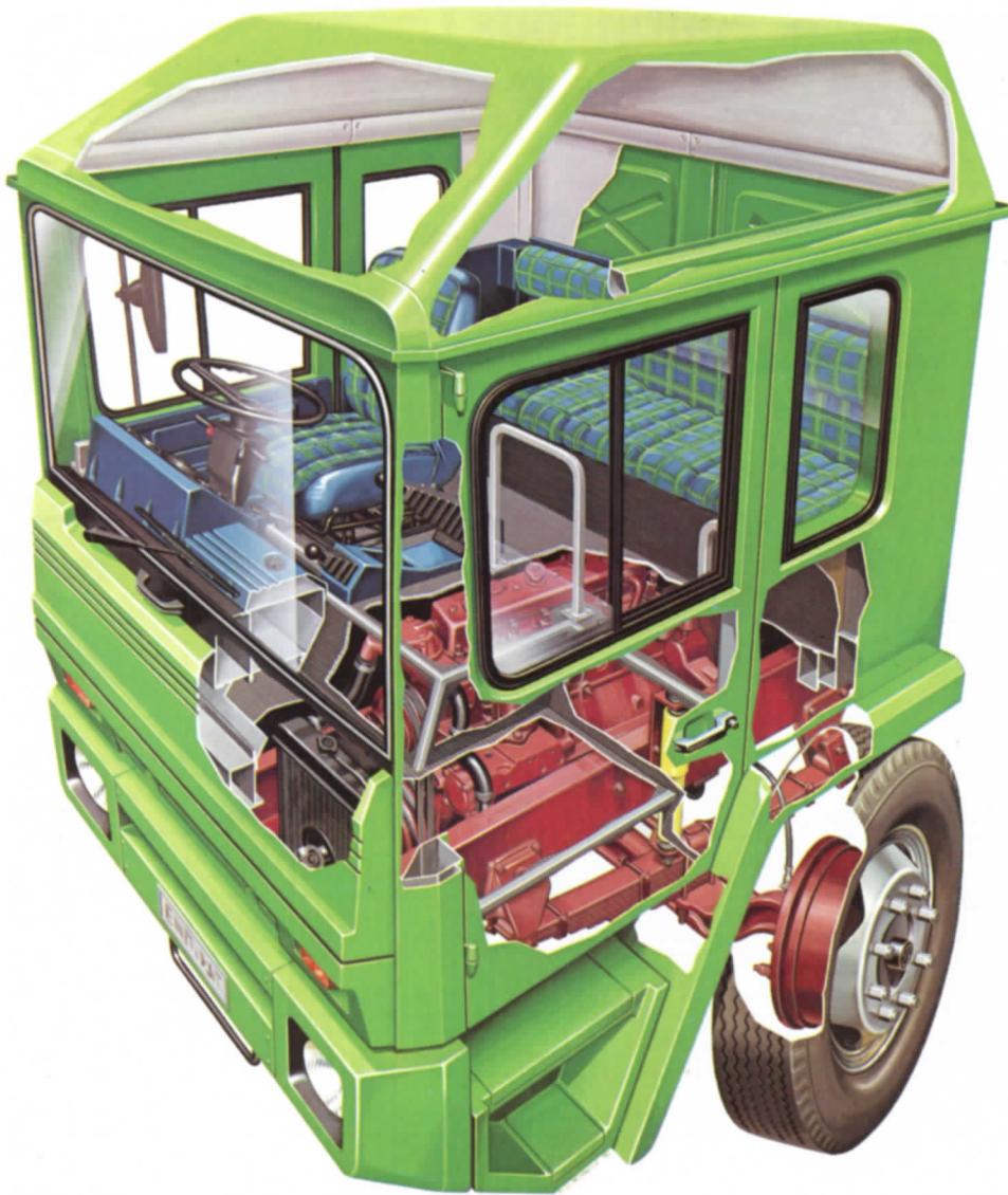
(left) This cut away view shows P Series strength of construction. Box section cantrails and side pillars give crew all round protection. Construction is all steel with certain non-structure panels in GRP for lightness. Power unit position allows obstruction free cross cab access with flat floor for fast crew entry/exit (below) P Series interior is fully trimmed with all driver's instruments easily visible through two spoke wheel. Additional controls are located in centrally mounted floor console. Fascia also contains fuse box access and storage space
