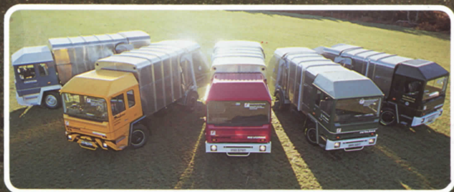
Shelvoke P Series, chassis across five GVW ranges, four cab versions, choice of two chassis widths
