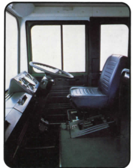
(left) This cut away view shows P Series strength of construction. Box section cantrails and side pillars give crew all round protection. Construction is all steel with certain non-structure panels in GRP for lightness. Power unit position allows obstruction free cross cab access with flat floor for fast crew entry/exit (below) P Series interior is fully trimmed with all driver's instruments easily visible through two spoke wheel. Additional controls are located in centrally mounted floor console. Fascia also contains fuse box access and storage space
