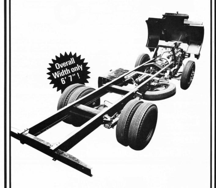
Model: NN series Tiltcab 11-5 tons (11684 kgs) GVW 4 x 2
