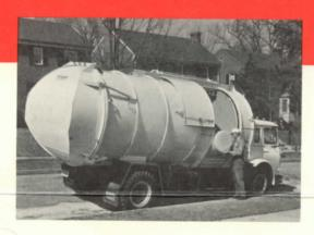
Truxmore Pakker—the King of the side loaders. With cylindrical construction, the body is cradled lower on the truck frame. This unit provides the lowest hand loading height of any side loading machine. The sills of the wide loading doors are only 15 inches above the chassis frame.
