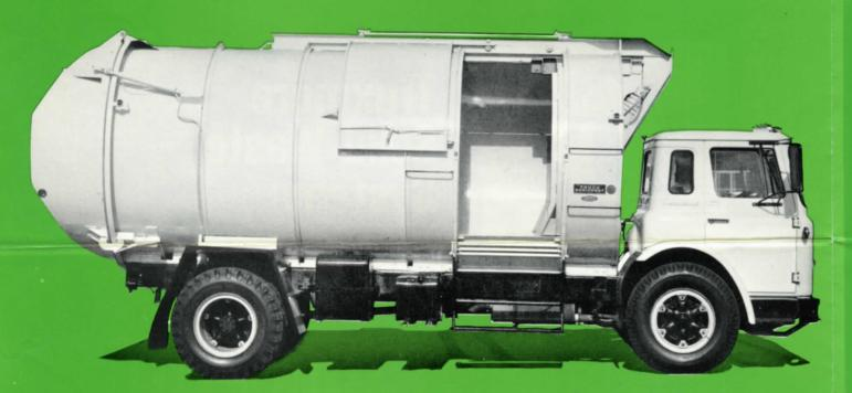
Wide loading doors on either side permit easy loading of boxes, crates, and tree limbs along with the normal refuse. The round body is cradled low on the truck chassis so the sills of the loading doors are only 15 inches above the frame. For maximum safety at the landfill, all of the controls for load ejection are located at the front of the body. The operator never has to risk going behind the Truxmore unit as he would have to do with trucks having doors that swing open to eject the load.
