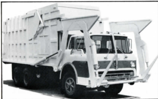
Front-end loaders— capacities 25 cu. yds. to 40 cu. yds.
