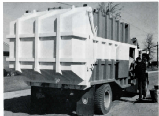
Side loader—capacity 22 cu. yds.
