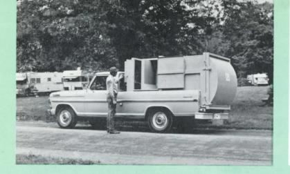
Simply open either side door, throw in the trash and watch the full traveling blade squash the material. An engine driven PTO powers the hydraulic pump to give 5 tons of blade force — and a complete cycle is only 15 seconds.
