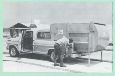
Need to use the pickup without the PUP? Just disconnect the hydraulic quick couplings and winch the PUP off on it's legs and the truck is free for any purpose. Takes about five minutes.
