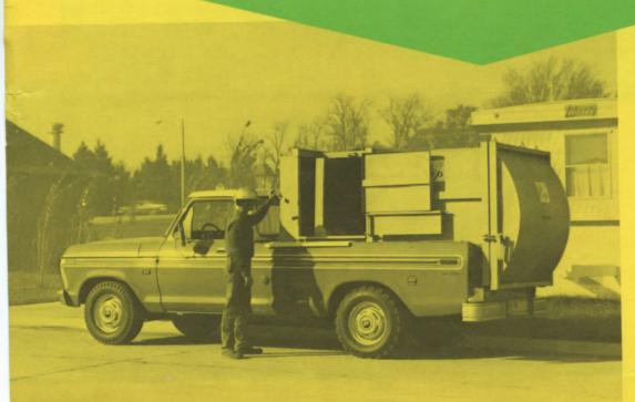
Simply open either side door, throw in the refuse and watch the full traveling blade pack the material. An engine drive PTO powers the hydraulic pump to give 5 tons of blade force and a complete cycle is only 15 seconds.
