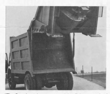
"The Gruncher takes excess weight off the rear axle of the vehicle. The proven Gruncher tailgate weighs considerably less than the conventional back-hoe type, allowing more payload per trip. For unloading, the Gruncher tailgate raises completely. The ejector blade unloads the body rapidly. Note the reinforced protection on the underside of the Gruncher's tailgate.'
