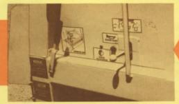
First time users are surprised at the number of "stops" that can be made in a given period of time. Non-stop or short-stop pickups are made possible by the **Gruncher** because the auger runs continuously along the route.
