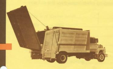
The **Gruncher** can be optionally equipped with cylinder powered container lifters for small containers (up to 3 cu. yd.) or overhead container lifters that exert a maximum pulling force of 10,000 pounds.
