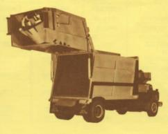
The **Gruncher** tailgate elevates completely and the clean smooth ejector blade empties the body in seconds. No time is wasted here.
