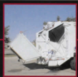
Cart dumper shown with optional winch
