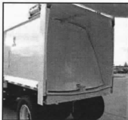
Curved Ejector Panel Cleanly ejects garbage
