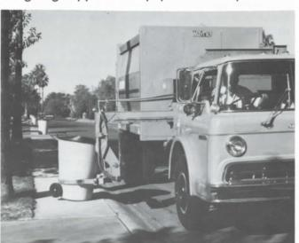
There's no unsightly clutter or disturbing clatter with polyethylene containers. Automated Curbtender meets EPA noise regulations with low power requirements and unique auger-type compaction.
