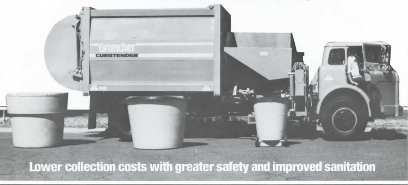
Curbtender<sup>™</sup> collection is faster than other equipment because of power arm's 6½-ft. extension. Operator can reach between parked cars and does not have to position truck precisely beside containers.
