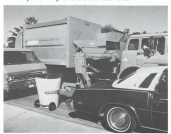
Curbtender Systems provide automated collection trucks and container options for curb, alley and commercial refuse collection. Customers receive assistance with evaluations, implementation, training and have access to on-going support for equipment and operations.
