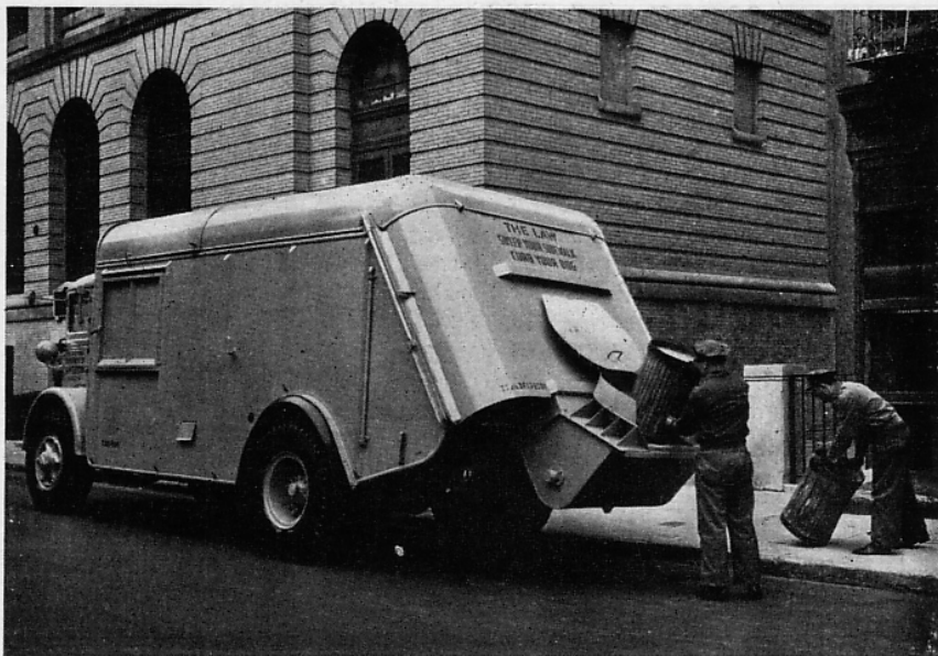
Loading the hopper of a late model New York City refuse truck. From the hopper refuse is conveyed into the truck body by hydraulically operated flights carried by chains somewhat like an escalator
