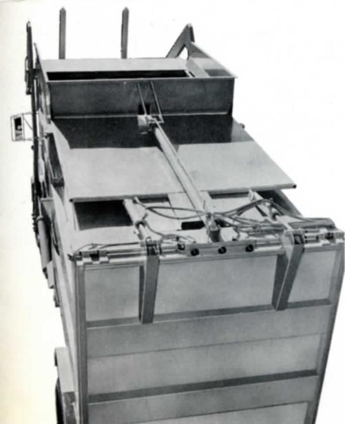
Hydraulic mechanism for hopper and rear front door (hopper door available in sliding or hinged style)
