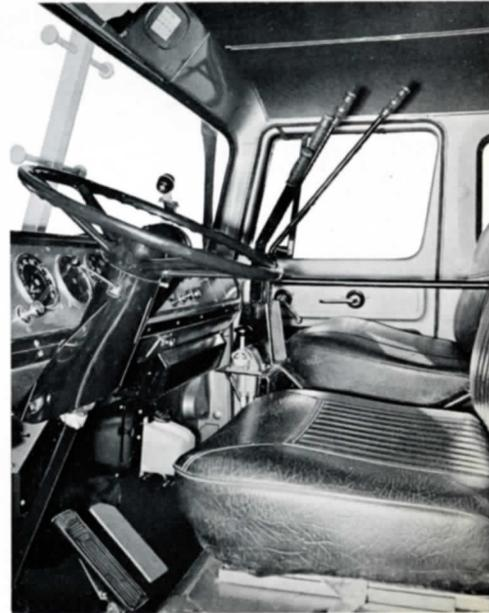
Driver controls showing windshield protection bar/ladder
