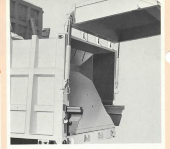
Twin cylinders raise and lower bubble tailgate. Platen moves out past body to insure complete ejection of the load.
