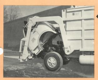
SERVICE ACCESSIBILITY—Cab tilts for service with lift arms down or raised. Hopper cover stays down when cab is tilted without making any disconnections.
