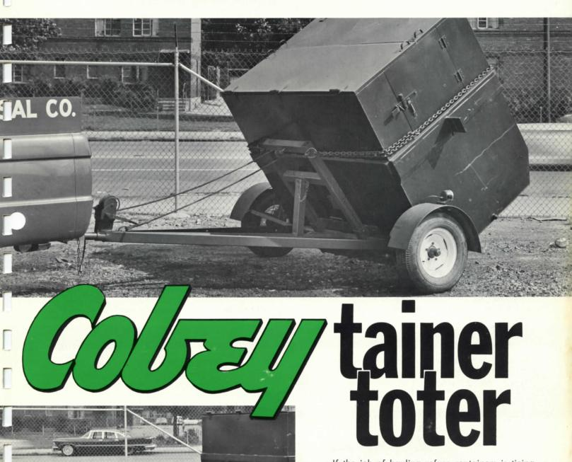
If the job of hauling refuse containers is tieing up valuable equipment (or ruining the bed of your pickup!), this rugged new gem from Cobey is for you! The "Tainer-Toter," a one-man two-wheeled unit, will even hitch up to an automobile, and will deliver your containers . . . anywhere! Perfect for your maintenance program, or delivery of new units.
