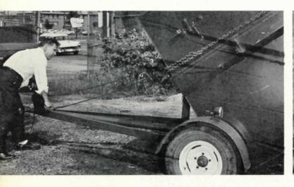
ONE-MAN OPERATION! Think of the hours and equipment saved! Fool-proof hand winch does the job, angles container properly for transport, lowers it safely at exact point of delivery.
