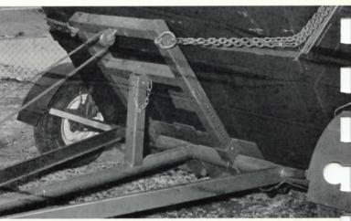
RUGGEDLY BUILT! Timken bearing equipped, 5-stud hubs, 11/2" cold roll steel spindles. Heavy duty lock pin and chain assembly holds container firmly in position. Flange adjusts for caster units.
