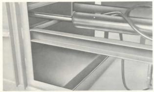
REDUCE ODOR AND FLY PROBLEMS—Design of the charging box floor flows liquids into the container... not on the ground! Mounted on legs, the SP-10 has lots of space underneath for easy cleaning to meet the most rigid inspection.
