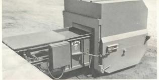
EASY TO INSTALL AND SERVICE—The SP-10 is completely self-contained. To install simply adjust leg height, anchor in place and connect to electric power line. There's no separate power pack to install! No chance of mistakes in wiring and plumbing! Saves dock space! All components are accessible from either side or by removing top cover.
