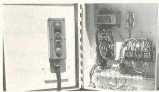
**ELECTRIC CONTROLS**—Plagued by 208 voltage? Deluxe electrical components are standard on the SP-10 to handle this and other common voltages without need for "special order equipment". All wiring is color and number coded. Weatherproof panel box.
