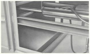
REDUCE ODOR AND FLY PROBLEMS—Design of the charging box floor flows liquids into the container... not on the ground! Mounted on legs the SP-20 has lots of space underneath for easy cleaning to meet the most rigid inspection.
