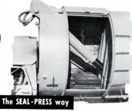
From inside the truck cab, with simple lever operation driver operates the driving of packing plate...to pack...or to eject. Tremendous pressure originates here at first stage of double acting, telescope type cylinder.
