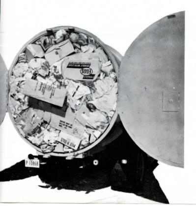
At the superior pressure of 85,000 lbs.\* a Seal-Press unit will compress a greater amount of refuse than one could imagine in such a compact unit. This means fewer trips to dump... greater payloads...lower operating costs. Comprehensive studies show that SEAL-PRESS units complete their run in fraction of time of other units.
