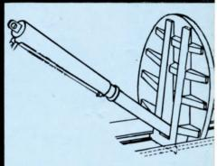
Here is close up of double-acting, telescope type multi-stage hydraulic cylinder which drives packing plate, after simple lever operation, to back of unit for most compact packing...or complete ejection.
