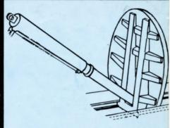
Here is close up of double-acting, telescope type multi-stage hydraulic cylinder which drives packing plate, after simple lever operation, to back of unit for most compact packing...or complete ejection.
