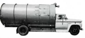
Loading Door Opening Width: 37 inches Oil Tank Capacity: 45 gals. Body Liquid Capacity: 500 gals. approx. Body Weight: 9,500 lbs. approx. O.D. of Main Cylinder: 91/4' O.D. of First Stage: 8 7/16" O.D. of Second Stage: 61/4" O.D. of Third Stage: 4 3/8" Total Stroke: 163 inches Loading Height Above Frame: 22 inches Total Compaction Force: Approx. 85,000 lbs. @ 1.500 PSI
