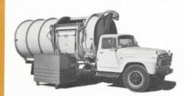
Photos show the quick, efficient operation. The container has been attached to the hoisting mechanism on the side of SEAL-PRESS refuse unit.
