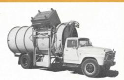
Container is carried quickly to top of refuse body and emptied into it. Hydraulic packing takes place, packing any type of refuse at 85,000 lbs.\*
